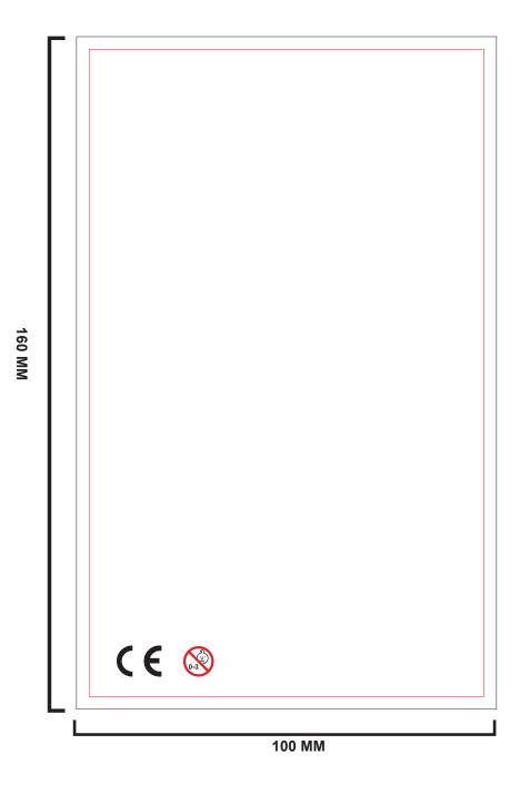
the cutting lines must be at least 3 mm distance from the art work
